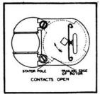
The contacts should open when the trailing edge of the rotor is approximately flush with the edge of the other stator pole.
